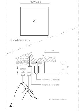
Note: The client is responsible for providing a robust 3/4" (19mm) plywood backing or wood blocking to securely anchor to the structural substrate.
