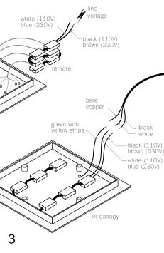
Connect transformers inside the canopy to line voltage. 110 V or 230 V depending on transformer.
