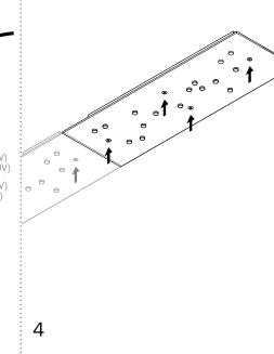
Anchor canopy into the plywood backing using the fasteners provided.
