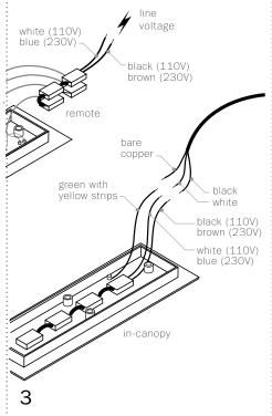
Connect transformers inside the canopy to line voltage. 110 V or 230 V depending on transformer.
